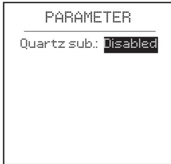
5. Quartz substitution allows the signal system to continue to operate following a communications loss. It utilizes quartz clock timing for synchronization between signals. Signals are not in communication when this mode is enabled.
