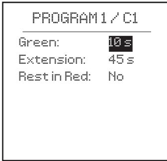
3. Set the green times for Phase 1. The first number on the screen is the base green. This is the minimum amount of green time a given phase will allow without detection. The second number is the extension time. The extension will only be applied if the system is using some form of vehicle detection. If you are not using detection, the extension will be ignored. Base green plus extension equals your maximum green time.
