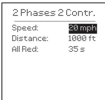
2. The speed of the work zone gets entered first, followed by the distance. The programmer uses these values to calculate a recommended All Red interval. This interval can still be adjusted using the Plus and Minus buttons.
