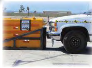
Inline TL-3 Truck Test Pre Impact
