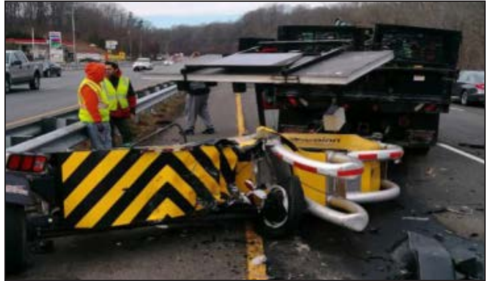
Scorpion attenuator struck by a VW Jetta at 80mph in Baltimore, MD. No serious injuries reported.
