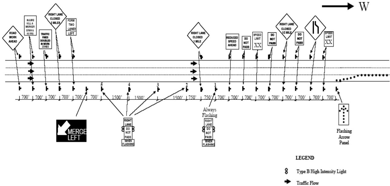
**Figure 2-** Dynamic Early Lane Merge Traffic Control System Used in Michigan (Source: Datta et al., 2004)
